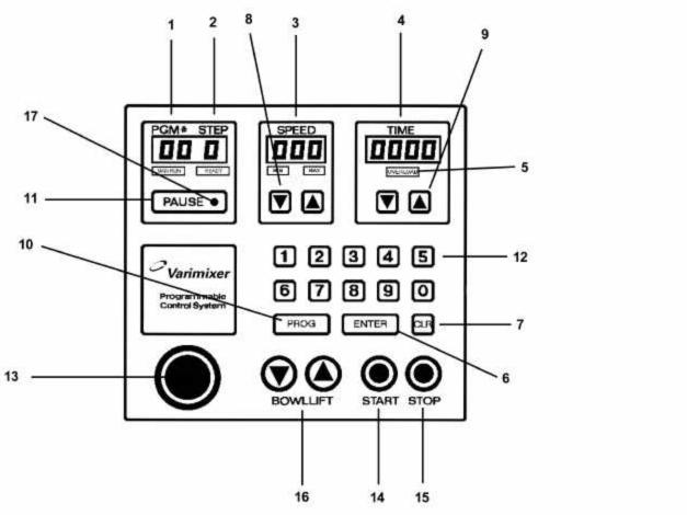
The Keypad is used for entering data to the system.
